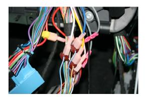
Here are the Orange and Green connectors that you had to blindly disconnect from the back of the CJB. Again, be sure to run the 3 wires behind the black metal bracket so they do not get pinched upon reassembly:
